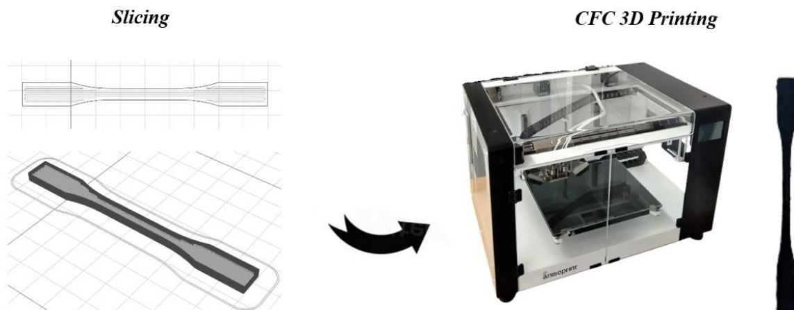
Fig. 2. Employed slicing strategy (left); Indicative images of Anisoprint Composer A3 3D printer and a 3D printed tensile specimen (right)
